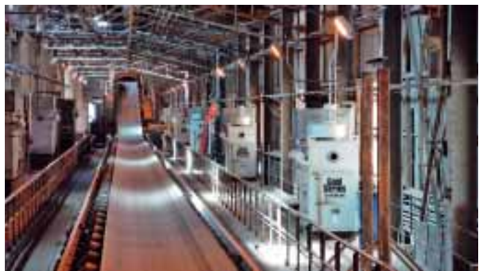
This Gold Series dust collector system supplied by Camfil Farr APC to a US copper mine offers high efficiency filtration through moisture-resistant HemiPleat® filters, "which offer greatly extended service life and lower pressure drop than standard pleated filters, the company says"
