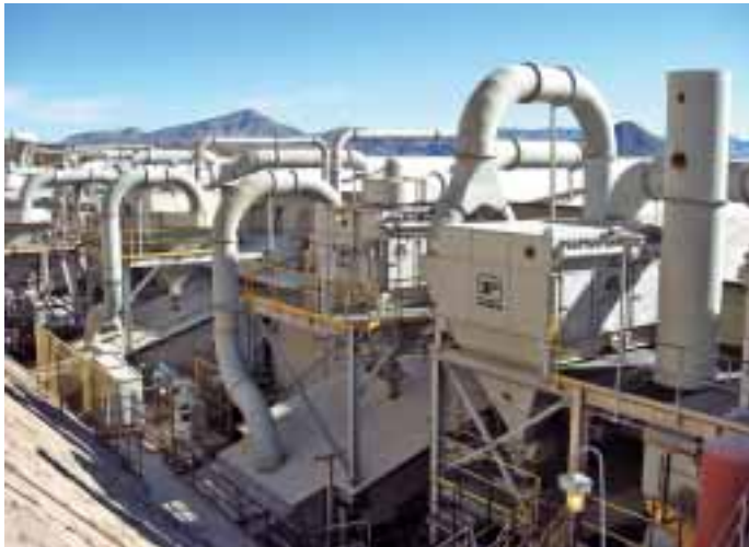
This Gold Series dust collector system supplied by Camfil Farr APC to a US copper mine offers high efficiency filtration through moisture-resistant HemiPleat® filters, "which offer greatly extended service life and lower pressure drop than standard pleated filters, the company says"
