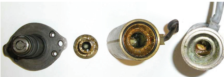
Before: Solenoid after 90 days use with previous fluid.
