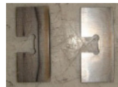
(Left) Excessive/premature vane wear.
