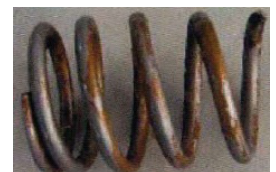
(Right) Example of the various areas of rust that were detected.
